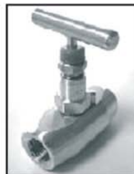
A65 Block Valve Body/Trim: 316Ti Packing: Graphite Rating: 2500lbs, 1/4"
