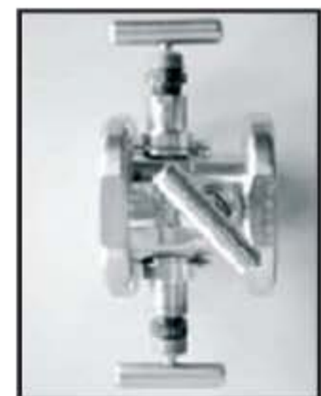
A66 3-Way Manifold Body/Trim: 316Ti Packing: PTFE Rating: 2500 lbs, 1/4"
