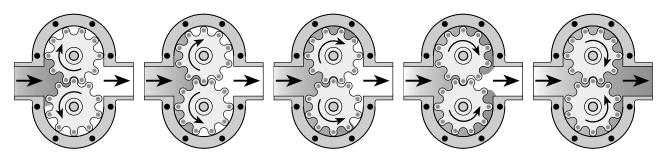
Flow Technology's positive displacement flowmeters use two rotating, thermoplastic impellers driven by the flowing liquid. Magnets imbedded in the impellers activate a non-intrusive sensor which generates a pulsed output signal. Each pulse represents a known volume of liquid that is captured in between the lobes of the impellers. A K-factor converts the pulses into engineering units for remote data collection and digital display.
